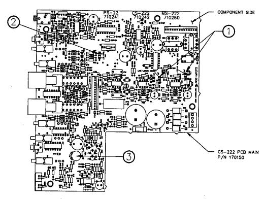
Location of Jumpers and Adjustments on PCB
